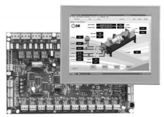
**DB DIRECTOR** in the DCLC chiller is complete with RS485 communications port and all hardware and software necessary to remotely monitor and control the packaged chiller up to 1500m away (hard wired).
