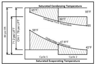
Referring to the above diagram, total refrigerant system lift is 84PSID. With DCLCT design and operation, total lift of Cycle #1 is reduced to 71.2PSID and for Cycle #2, it is reduced to 78PSID.
